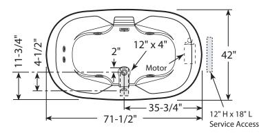
Product Shown: Fresco® Whirlpool Bath Right Hand Shown Model: BM90 \* Measurements inside unit represent cutout in floor to allow for drain/overflow. Minimum Service Access dimensions given.
